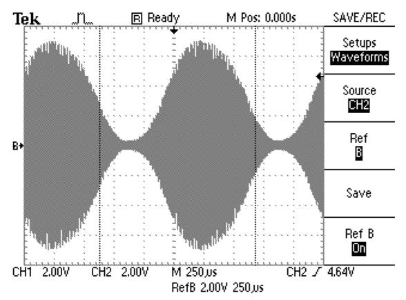
ZC1 Mk2 with ZL2TBH mods - 3.85 MHz with 800 Hz audio at level 8 mV
