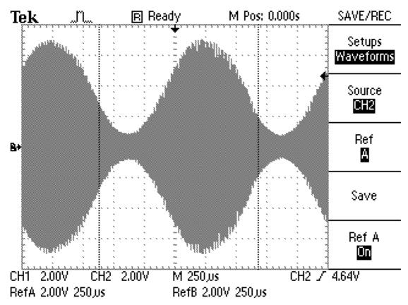
ZC1 Mk2 with ZL2TBH mods - 3.85 MHz with 800 Hz audio at level 6.3mV
