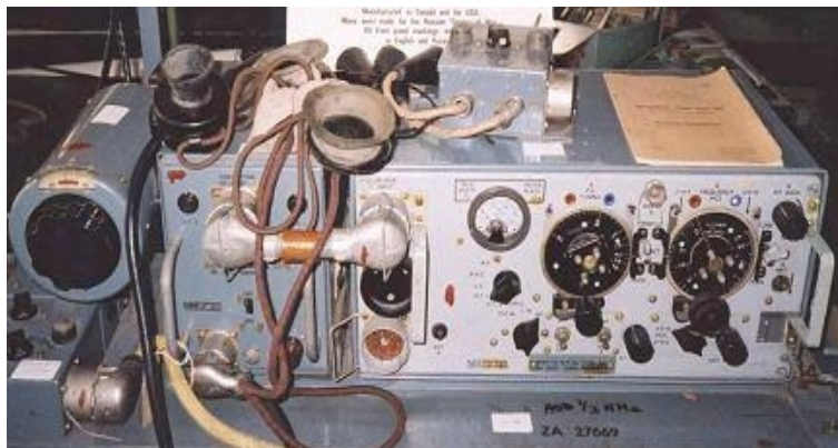
Wireless Set 19 – HF and VHF operation plus crew intercom.
