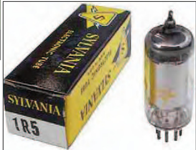
The original miniature tubes, designed for use in battery portables, had 1.4-volt filaments. This is the 1R5 pentagrid converter.
