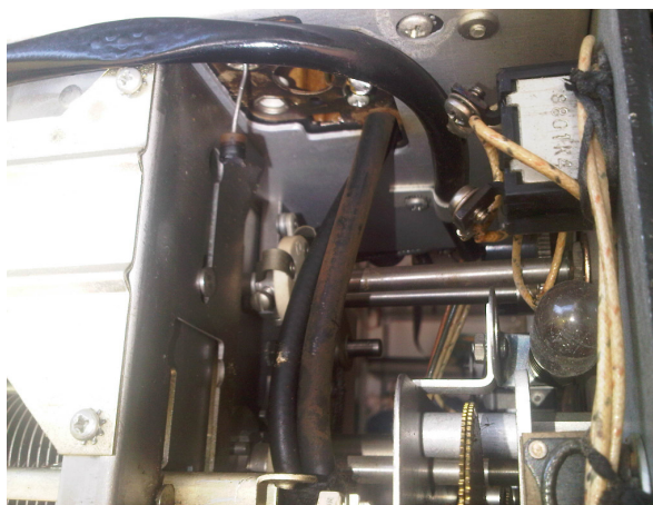
Coil can removed with remains of burnt resistor
