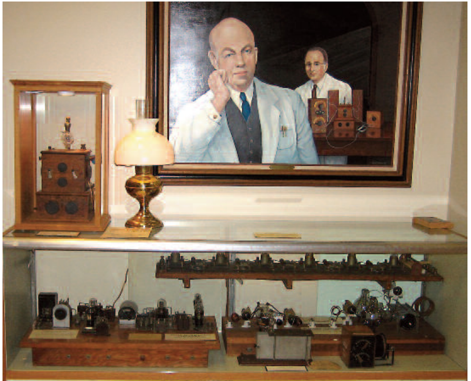
A display of Edwin Armstrong's actual laboratory equipment at the Antique Wireless Museum. It includes the 1914 patent model of his regenerative receiver (small case) as well as his superheterodyne circuit and Empire State Building FM transmitter (large case).
