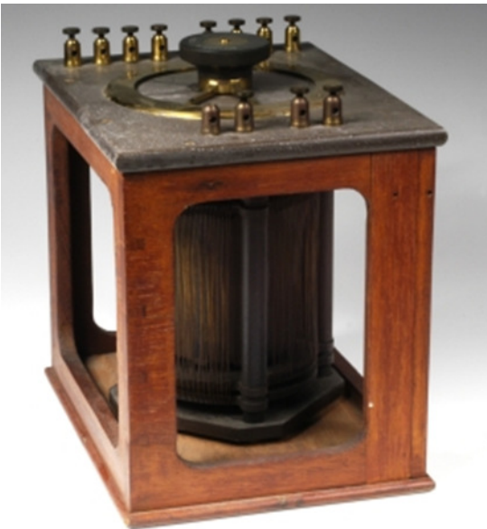
Marconi Bellini-Tosi Direction Finder, by Marconi's Wireless Telegraph Co. Ltd, c.1916. Marconi Collection
