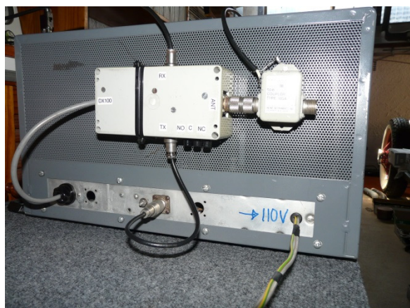
The arrangements for the 75A4 require a +20 volts DC for muting.
