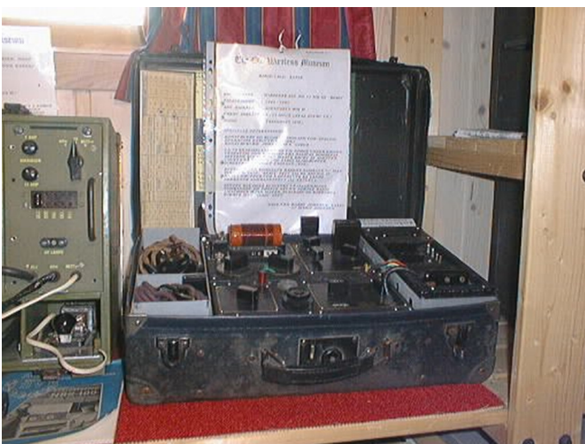
3MkII "Berit" Suitcase Radio, 16-20 Watts output, making this the most powerful of the SOE suitcase sets
