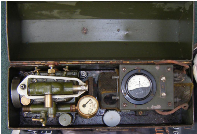
Alco Power Generator in carry case, was a steam generator heated by wood or coal
