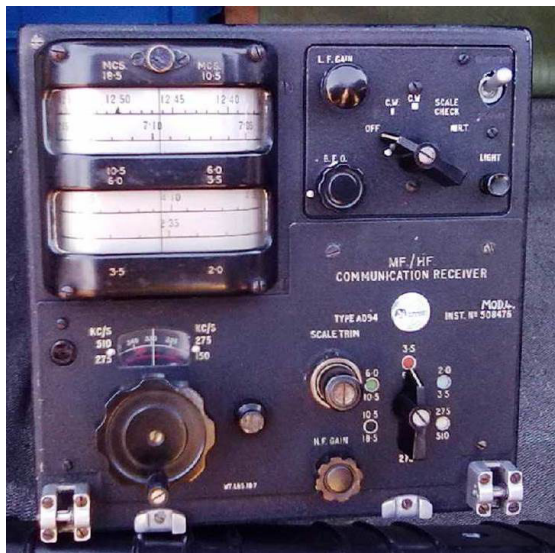
The Marconi AD94 HF communication receiver, a 12 valve superhet with a 30 foot direct reading film scale covering 150 to 510kHz and 2 to 18.5MHz
