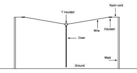
Figure 7 Dipole diagram showing sag due to coax
