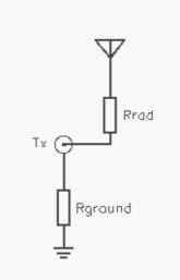
Figure 11 Vertical antenna
