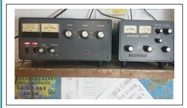
The Yaesu FL-2100Z is a classic HF amplifier. It sits near the end of a long life line of multiple variations and models of the basic 811A or 572B triode valve, all using exactly the same grounded-grid core design, and all of them making nice big waves in the ether.
