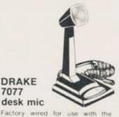
Factory wired for use with the TR7/DR7 modes push-to-talk or VOX dynamic, high impedance, frequency response 300-5000 Hz, output -48 dB at 1 KHz (0 dB=1V/microbar), 4 pin connector.
