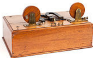
Magnetic detector by Marconi used during the experimental campaign aboard a ship in summer 1902, exhibited at the Museo nazionale della scienza e della tecnologia Leonardo da Vinci of Milan.
