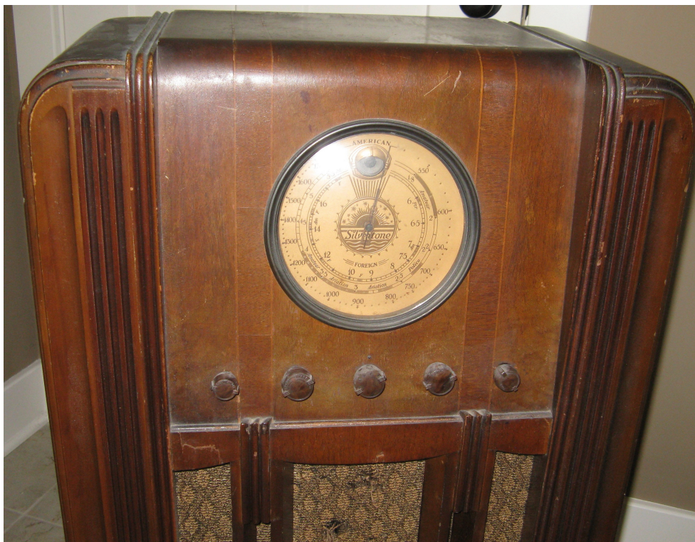
This photograph of the author's 1937 Silver-tone shows the markings for police, foreign, and amateur frequencies that were common on many radios during the 1930s
