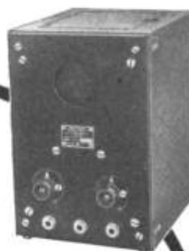
Type DA Detector Am- plifier, Style 307190, 2- stage, 3 tubes, Audio Frequency
