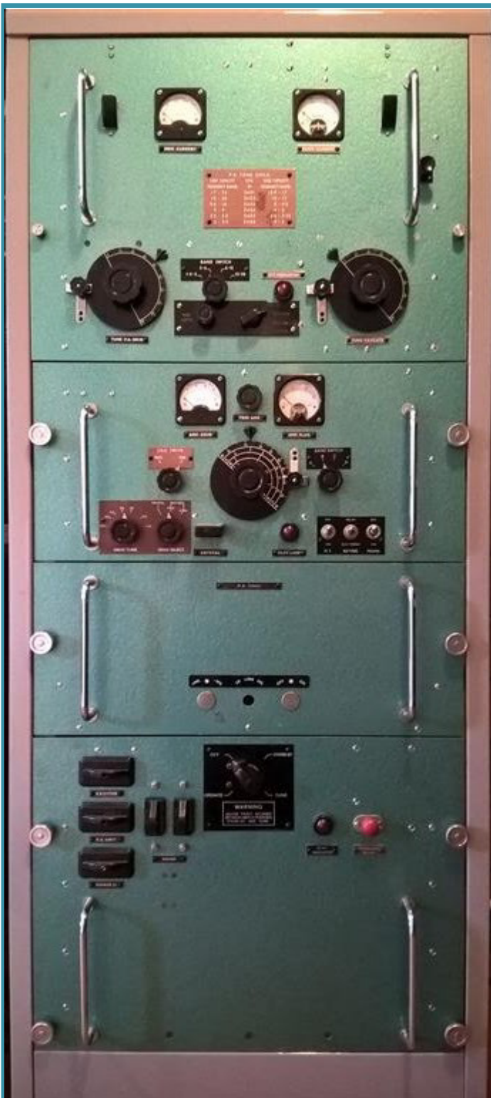
Fig 1. Diplomatic Wireless Service MK. 214D transmitter. This is SN161. The exciter top view photo is rotated in such a way that the panel front is on the right-hand side. The tube to the left top-side is an 807 (buffer amplifier) and the tubes in the bottom right-hand section are the oscillator (EF91) and the multiplier (EF55).
