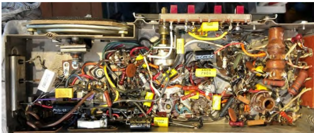
Photo right—Chassis that has been refurbished, ie all paper and electrolytic capacitors (yellow and black coloured parts) plus out of tolerance resistors replaced with modern components.
