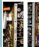
Next are two views of the left side and right side respectively, with some colored arrows pointing out most of the screws. The blue arrow in the second photo marks the wire mentioned in the next step.
