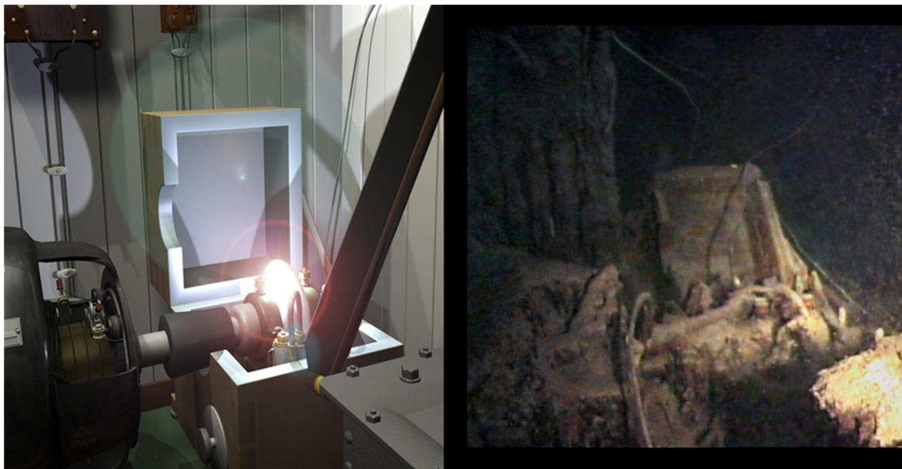
Above left: The disk discharger spark gap sat inside a teak box which served as a sound deadener. The lid of this box is in the open position (CGI by Parks Stephenson). Above right: The disk discharger transmitter as seen in 2019. It is believed that the lid was left open by radio operator Harold Bride. Photo by Earthship Productions
