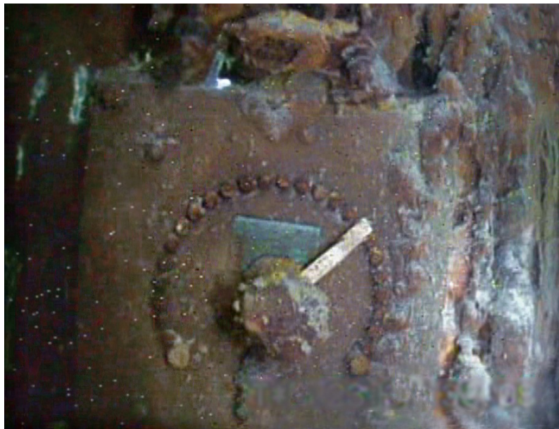
Above: One of the multi-tapped regulator boxes whose selector handle is shown in the exact position when Titanic sank. Photo by Earthship Productions
