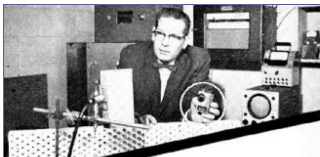
A dosimeter developed by Dr. A. W. Richardson of Saint Louis University is used to measure r.f. radiation. Worn by a maintenance technician, it sounds an audible tone when r.f. intensity becomes dangerous.
