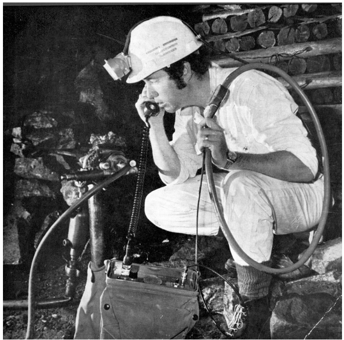
Figure 5: The single-sideband 335 kHz solid-state transceiver with its
